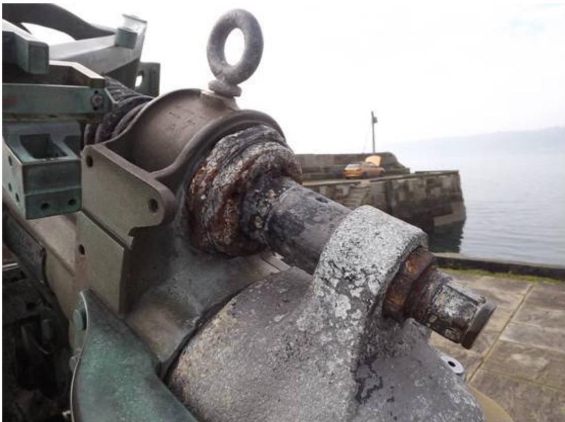
*Plate 63 Vincent's Pier, detail of Vickers breech mechanism*
