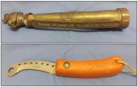
Above are two donations from Mr Peter Baker. The top image is a brass Dobbie-McInnes Depthometer made in Glasgow. Above is an RAF Dingy knife with a cork handle so it stays afloat if dropped in the water. It has a rounded end so it does not puncture the dingy!
